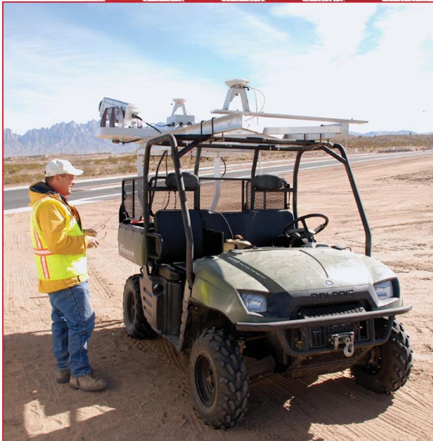
An exchangeable platform holding all of the LYNX system's components allows WHPacific the versatility to conduct a four-mile cross country waterline design survey.
