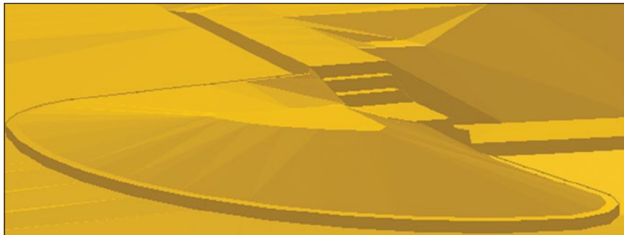
Figure 6 Rendered “as-built” surface showing good demarcation of curbs, steps and pavement slopes
