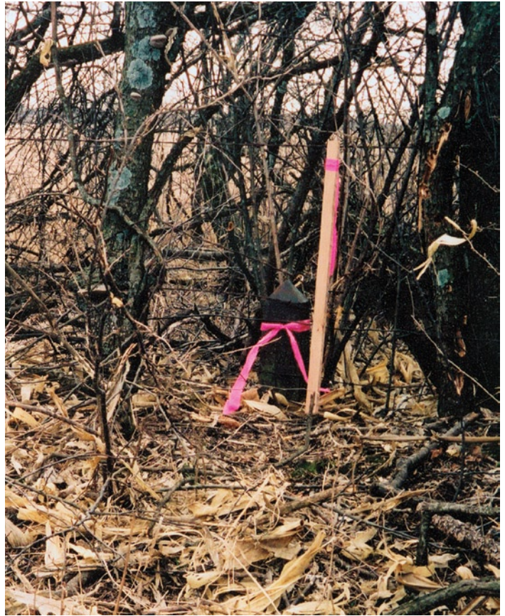
Mile 60 East was recovered along a heavily wooded fence line utilizing search positions entered into a Trimble Geo-Explorer handheld GPS unit.
