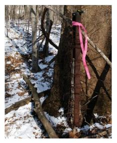
This found railroad rail ostensibly marks the position of a stone property corner set March 23, 1886. In 1943, an "iron corner post" was set in the same location. Was the railroad rail one and the same as the "iron corner post?" The surveyor in 1886 had also set a stone as a witness 2 rods to the north.
