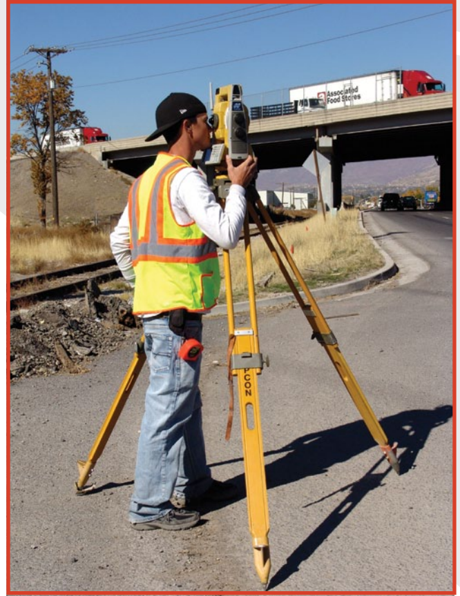
Dave Norman back-sights a control point to set up his robotic total station.
